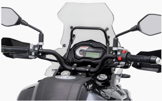
TRK 502 X features a large headlight fairing that guarantees maximum protection, handguards with aluminum insert and customized with the motorcycle logo and a central stand. The handlebar, updated, is adjustable to allow each rider the best riding condition, as well as the clutch lever, which is also adjustable. It also features backlit handlebar switchgears, rear-view mirrors with new design, as well as the new hand grips and practical aluminum pawls positioned under the saddle, comfortable and
